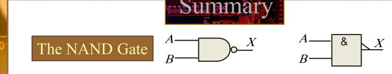
The NAND gate produces a LOW output when all inputs are HIGH; otherwise, the output is HIGH. For a 2-input gate, the truth table is \_\_\_\_\_\_\_
