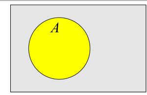
The diagram visually shows that A + AB = A. Other rules can be illustrated with the diagrams as well.
