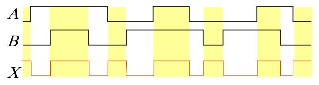
Notice that the XNOR gate will produce a HIGH when both inputs are the same. This makes it useful for comparison functions.
