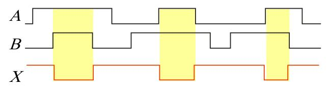
The NAND gate is particularly useful because it is a "universal" gate – all other basic gates can be constructed from NAND gates.
