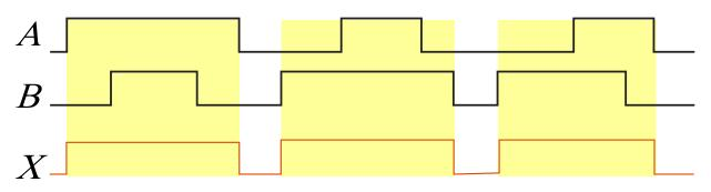
The OR operation can be used in computer programming to set certain bits of a binary number to 1.
