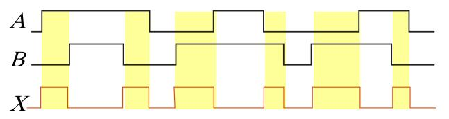
Notice that the XOR gate will produce a HIGH only when exactly one input is HIGH.
