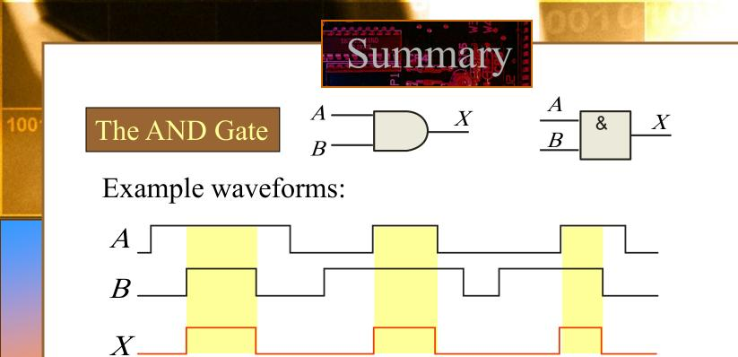
The AND operation is used in computer programming as a selective mask. If you want to retain certain bits of a binary number but reset the other bits to 0, you could set a mask with 1's in the position of the retained bits.
