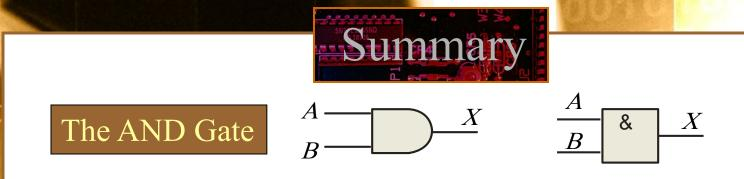
The **AND** gate produces a HIGH output when all inputs are HIGH; otherwise, the output is LOW. For a 2-input gate,
